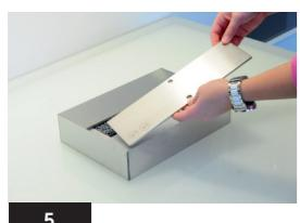
place the extinguisher sliding gauges on the combustion chamber. the extinguisher slide without the holes should be facing away from you.
