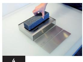
place the combustion sponge in the combustion chamber.
