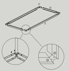
NB! Make sure the holes on the corner (C) are facing up.
