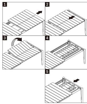
${\bf NOTE: BEFORE\ DISMANTLING, UNLOCK\ ON\ UNDERSIDE\ OF\ TABLE}$
